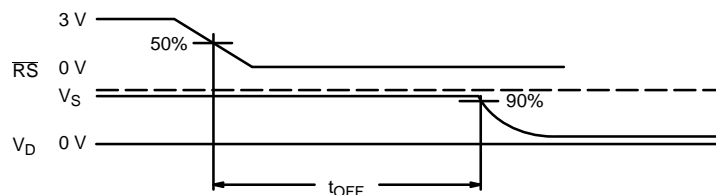
FIGURE 3. t_{OFF} from \overline{RS}
