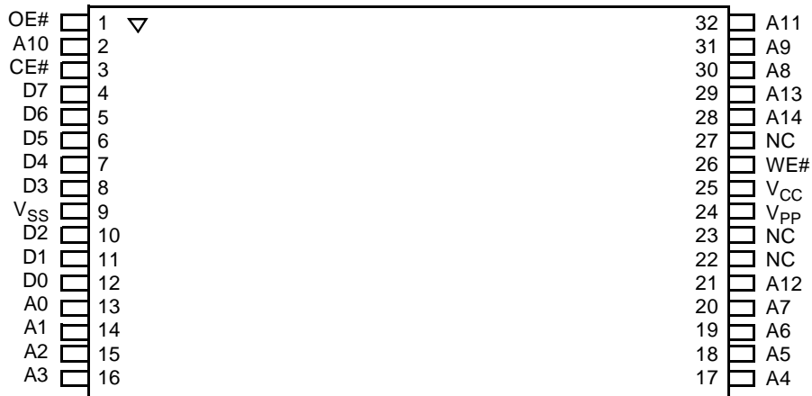
32-Pin TSOP—Reverse Pinout
