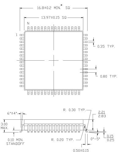
64-Lead Ceramic Quad Flatpack (Cavity Up) U65
