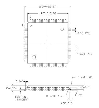
DIMENSIONS IN MILLIMETERS LEAD COPLANARITY 0.102 MAX.
