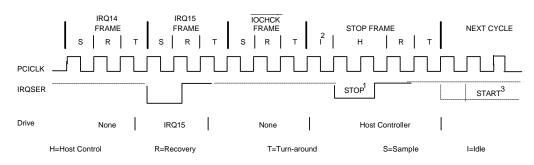
1. Stop pulse is 2 clocks wide for Quiet mode, 3 clocks wide for Continuous mode.
