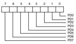
The contents of DB0-DB7 are buffered (non-inverting) and output to ports PD0-PD7 during a write operation. The leading edge of  $\overline{IOW}$  causes an EPP address write cycle to be performed, and the trailing edge of  $\overline{IOW}$  latches the data for the duration of the EPP write cycle.
