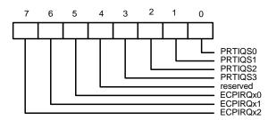
ECPIRQx2-ECPIRQx0 (Bit7-bit 5): These bits are configurable equivalents to bit[5:3] of cnfgB register in ECP mode, except that cnfgB[5:3] are read-only bits. They indicate the IRQ resource assigned for the ECP printer port. It is the software designer's responsibility to ensure that CR27[7:5] and CR27[3:0] are consistent. For example, CR27[7:5] should be filled with 001 (select IRQ 7) if CR27[3:0] are to be programmed as 0101 (select IRQ\_E) while IRQ\_E is connected to IRQ 7.
