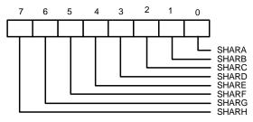
This register is used to select whether these interrupt request pins are in the IRQ sharing mode. While in the IRQ sharing mode, the corresponding pin is low active for 200ns for the interrupt request and keeps tri-stated otherwise.
