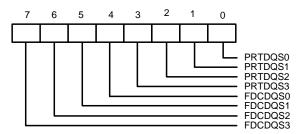
FDCDQS3-FDCDQS0 (Bit 7-bit 4): Allocate DMA resource for FDC.
