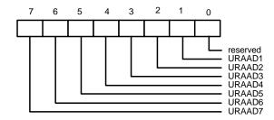
This register is used to select the base address of the UART A from 100H-3F8H on 8-byte boundaries. NCS = 0 and A10 = 0 are required to access the UART A registers. A[2:0] are don't-care conditions.
