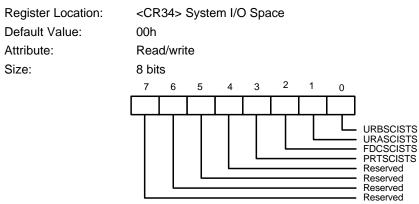
These bits indicate the status of the SCI input, which is set when the device's IRQ is raised. If the corresponding enable bit in the SCI interrupt enable register (in GP0EN1) is set, an SCI interrupt is raised and routed to the output pin. Wrinting a 1 clears the bit, and writing a 0 has no effect. If the bit is not cleared, new IRQ for the SCI logic input is ignored, therefore no SCI interrupt is raised.
