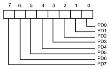
When accesses are made to any EPP data port, the contents of DB0-DB7 are buffered (non-inverting) and output to the ports PD0-PD7 during a write operation. The leading edge of  $\overline{IOW}$  causes an EPP data write cycle to be performed, and the trailing edge of  $\overline{IOW}$  latches the data for the duration of the EPP write cycle.
