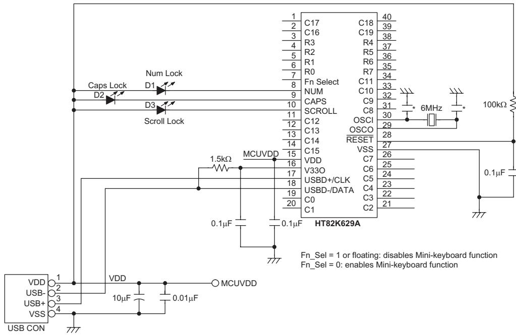
Note: For single side PCB, the GND should be routed first. Avoid routing the GND line and VDD line with jumping wires.
