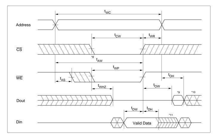
Write Timing Waveform (2) (OE Low Fixed)
