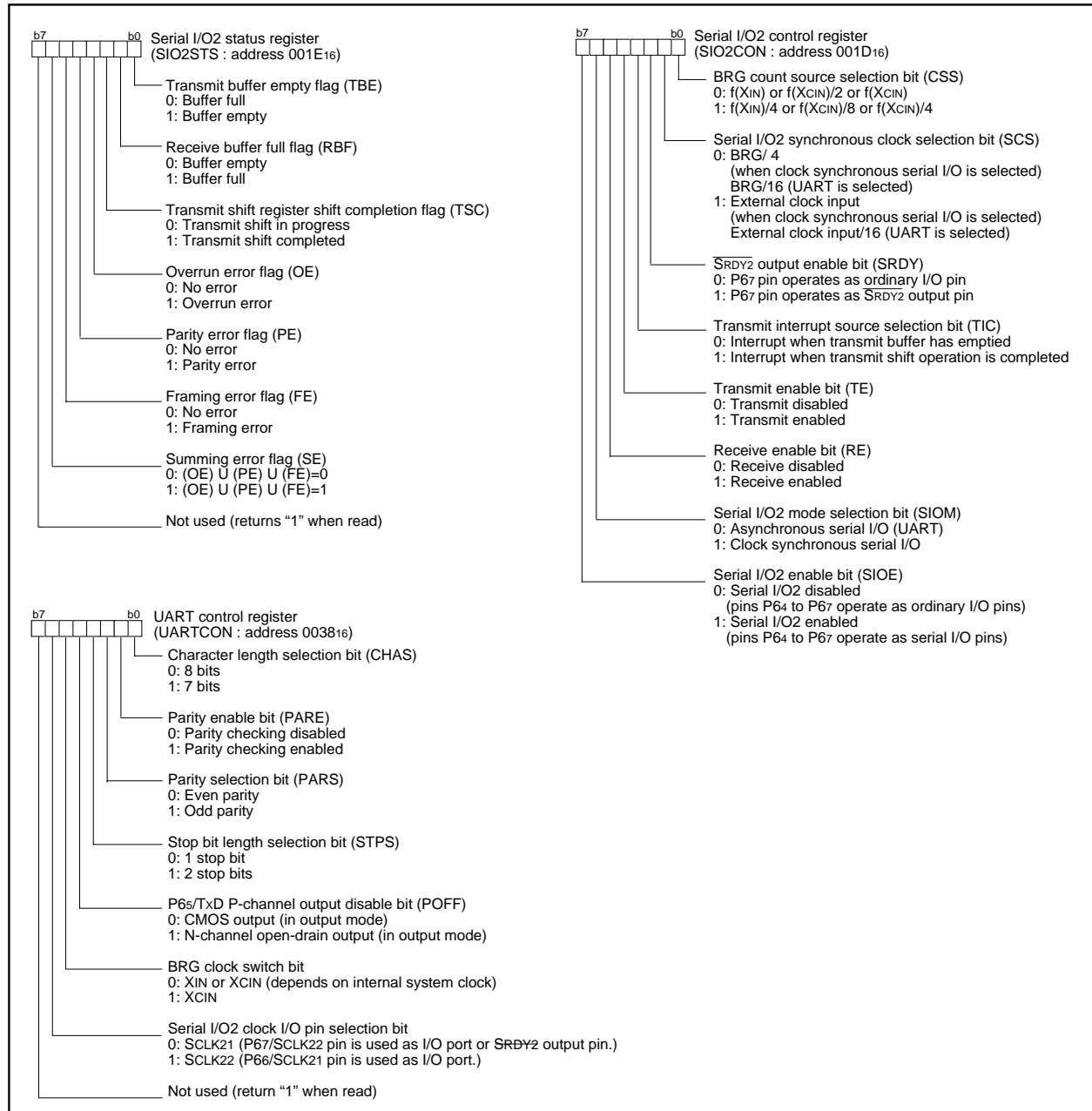
Fig. 40 Structure of serial I/O2 related register
