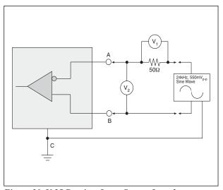
Figure 30. V.35 Receiver Input Source Impedance
