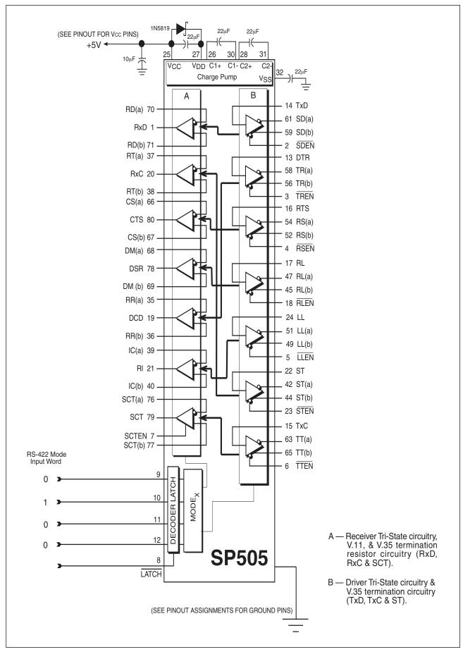
Figure 52. SP505 Typical Operating Circuit
