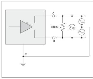
Figure 16. V.11 and V.35 Driver Output Open-Circuit Voltage
