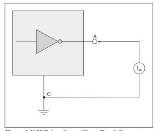
Figure 4. V.28 Driver Output Short-Circuit Current
