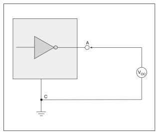
Figure 1. V.28 Driver Output Open Circuit Voltage
