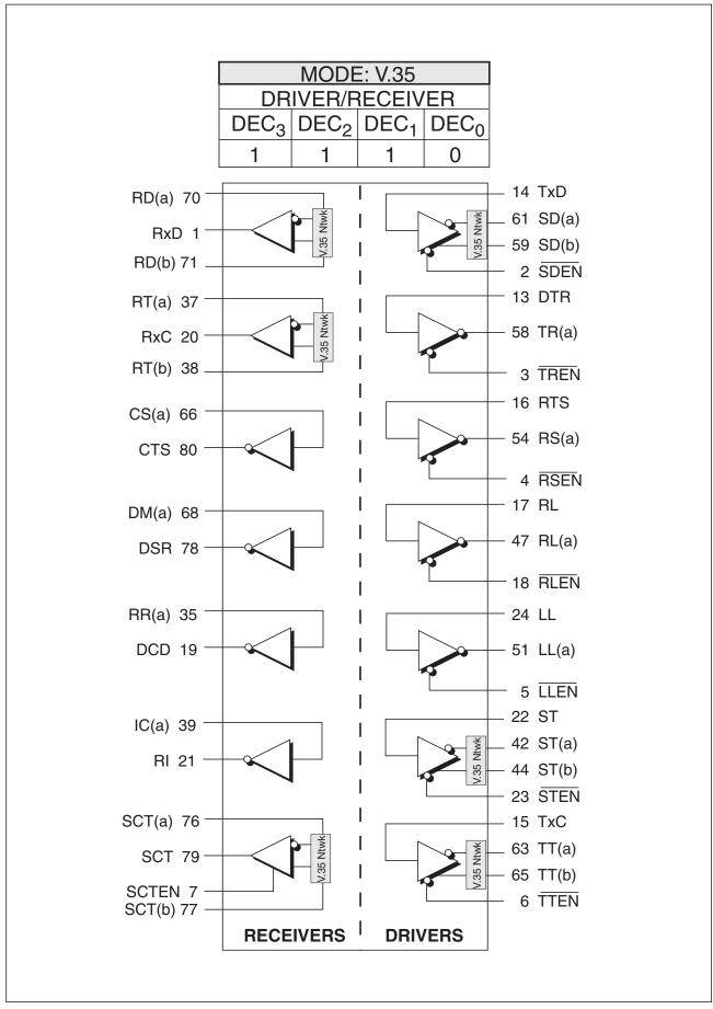
Figure 54. Mode Diagram — V.35
