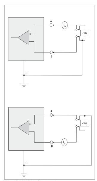
Figure 20. V.11 Receiver Input Current
