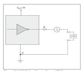
Figure 12. V.10 Driver Output Power-Off Current
