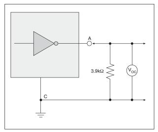
Figure 9. V.10 Driver Output Open-Circuit Voltage
