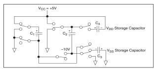
Figure 47. Charge Pump Phase 2 for +10V.
