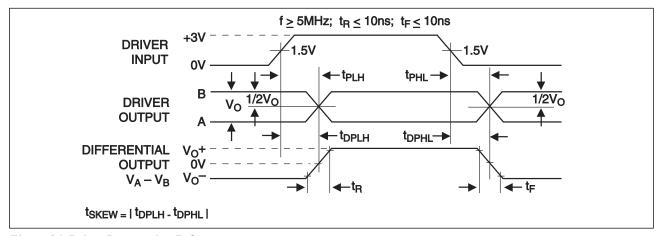
Figure 36. Driver Propagation Delays
