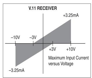
Figure 22. V.11 Receiver Input IV Graph
