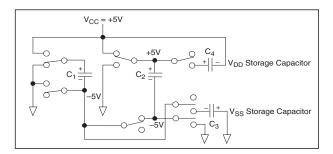
Figure 45. Charge Pump Phase 1 for  $\pm 10V$ .
