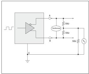
Figure 21. V.11 Driver Output Rise/Fall Time
