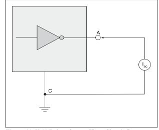
Figure 11. V.10 Driver Output Short-Circuit Current
