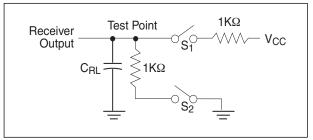
Figure 34. Driver Timing Test Load Circuit
