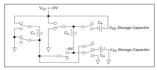
Figure 48. Charge Pump Phase 2 for  $\pm 5V$ .
