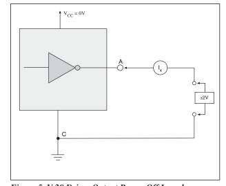
Figure 5. V.28 Driver Output Power-Off Impedance
