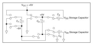
Figure 46. Charge Pump Phase 1 for ±5V.
