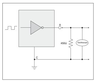
Figure 13. V.10 Driver Output Transition Time
