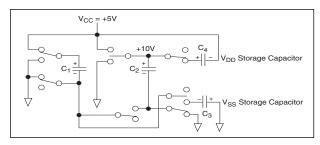
Figure 50. Charge Pump Phase 4.
