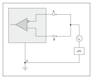
Figure 31. V.35 Receiver Input Short-Circuit Impedance
