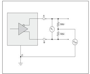
Figure 26. V.35 Driver Output Offset Voltage
