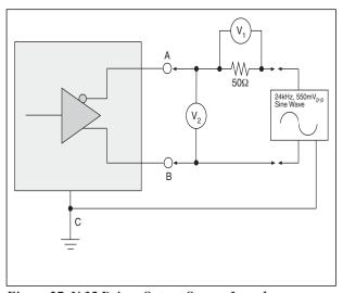
Figure 27. V.35 Driver Output Source Impedance
