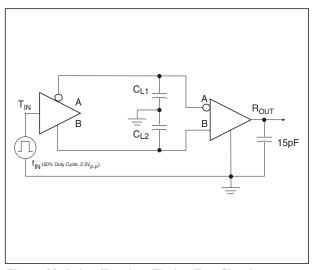
Figure 33. Driver/Receiver Timing Test Circuit
