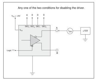
Figure 32. Driver Output Leakage Current Test
