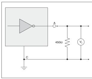
Figure 10. V.10 Driver Output Test Terminated Voltage
