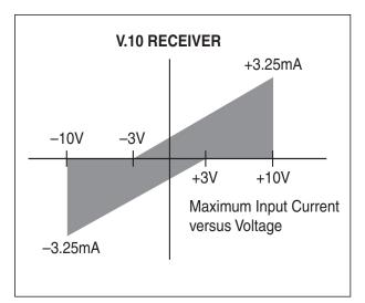
Figure 15. V.10 Receiver Input IV Graph
