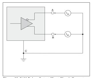
Figure 18. V.11 Driver Output Short-Circuit Current
