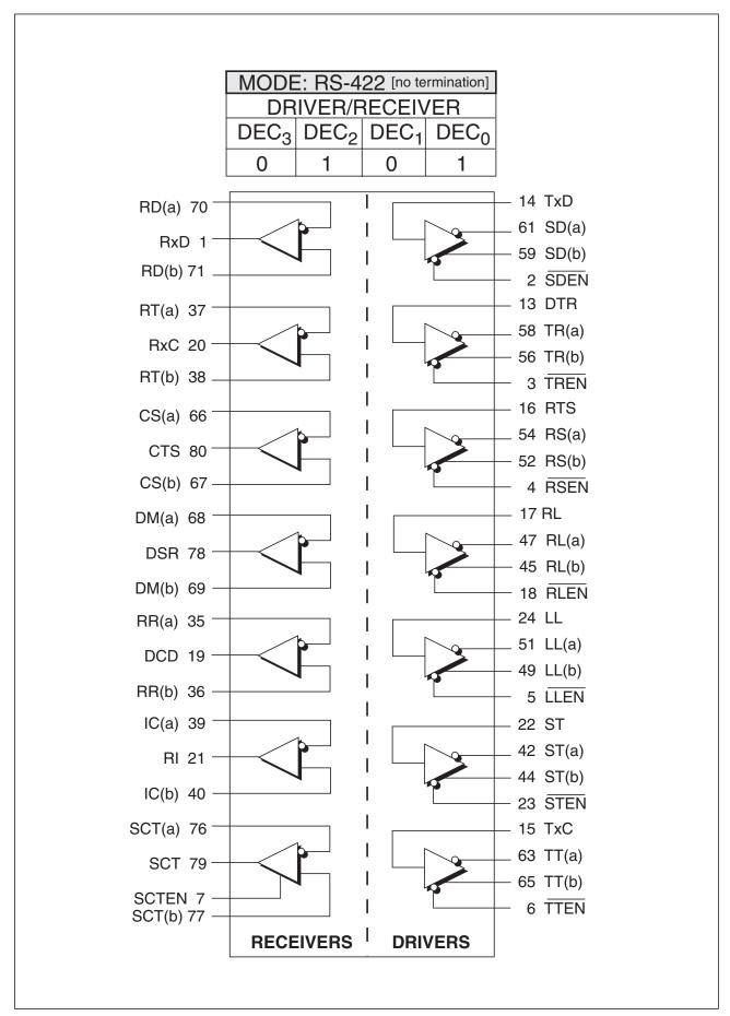
Figure 57. Mode Diagram — RS-422 w/o termination
