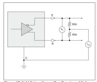
Figure 17. V.11 Driver Output Test Terminated Voltage
