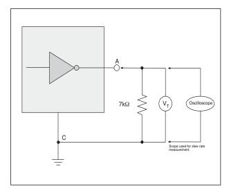
Figure 3. V.28 Driver Output Slew Rate
