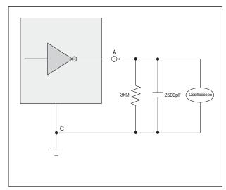
Figure 6. V.28 Driver Output Rise/Fall Times
