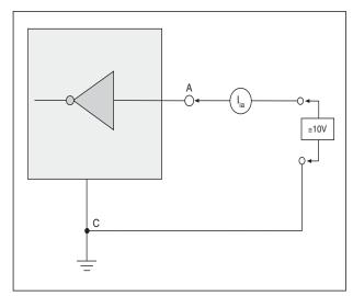
Figure 14. V.10 Receiver Input Current
