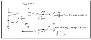
Figure 49. Charge Pump Phase 3.
