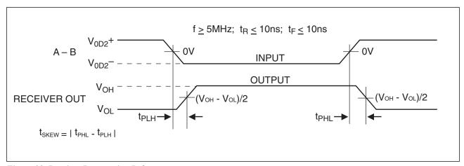
Figure 38. Receiver Propagation Delays
