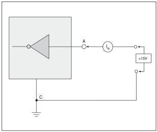
Figure 7. V.28 Receiver Input Impedance
