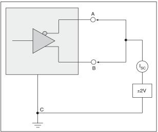
Figure 28. V.35 Driver Output Short-Circuit Impedance
