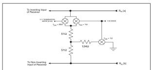
Figure 51. Simplified R<sub>IN</sub> Termination Circuit
