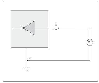
Figure 8. V.28 Receiver Input Open Circuit Bias
