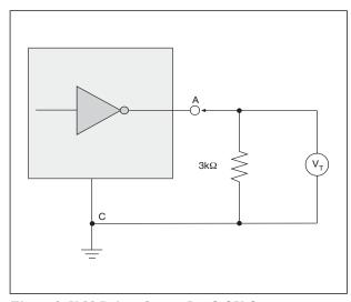
Figure 2. V.28 Driver Output Loaded Voltage
