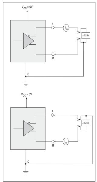
Figure 19. V.11 Driver Output Power-Off Current
