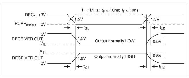
Figure 39. Receiver Enable and Disable Times
