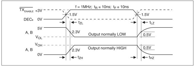
Figure 37. Driver Enable and Disable Times
