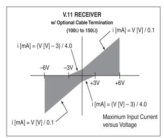
Figure 24. V.11 Receiver Input Graph w/ Termination
