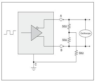
Figure 29. V.35 Driver Output Rise/Fall Time
