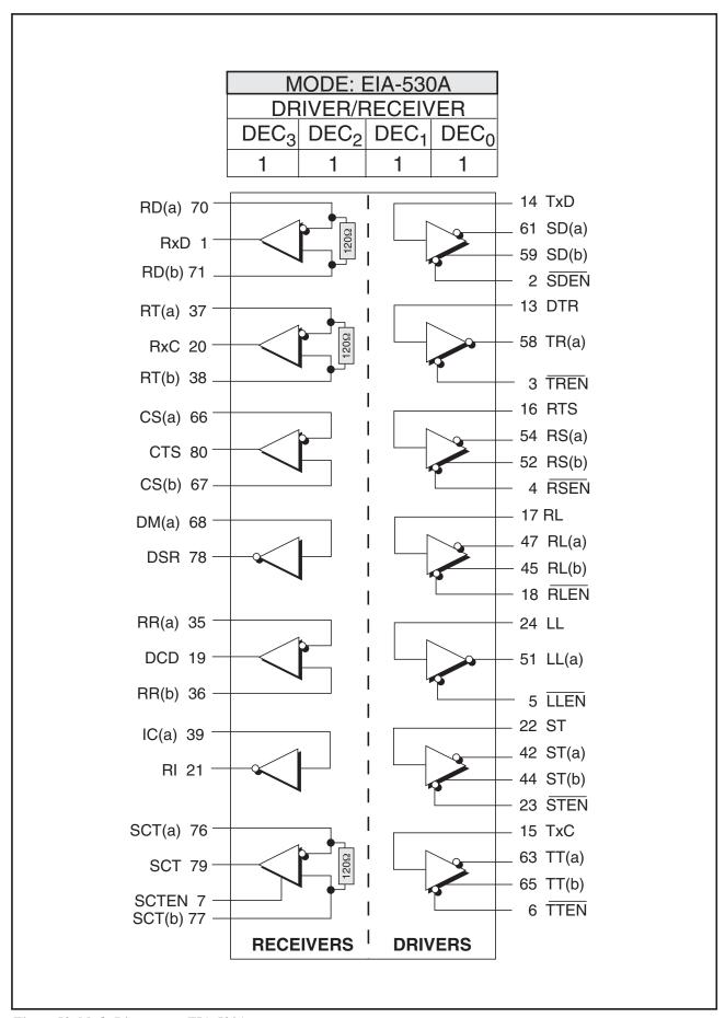
Figure 59. Mode Diagram — EIA-530A
