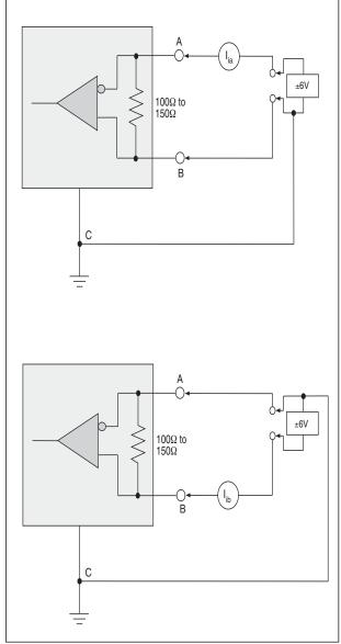
Figure 23. V.11 Receiver Input Current w/ Termination
