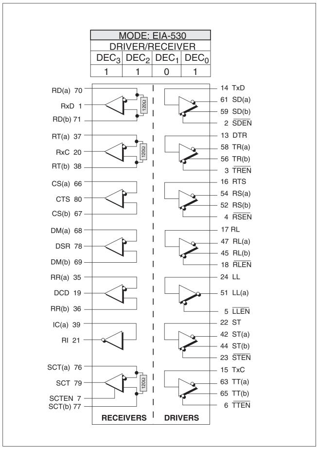
Figure 58. Mode Diagram — EIA-530
