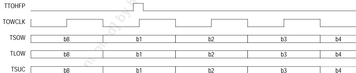
Figure 52 -TSOW, TLOW and TSUC Alignment w.r.t TTOHFP (TX_GAPSEL=0)
