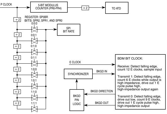
Figure 10-13. Clock Chain for SPI, ATD, and BDM
