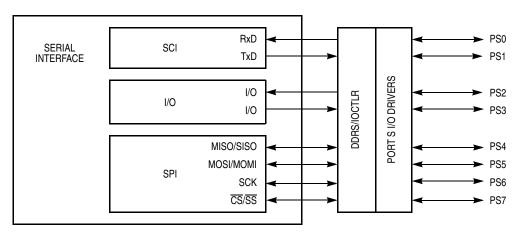
Figure 14-1. Serial Interface Block Diagram
