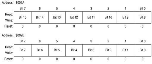
Figure 12-21. Timer Input Capture/Output Compare Register 5 (TC5)
