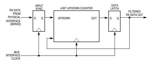
Figure 15-3. BDLC Rx Digital Filter Block Diagram
