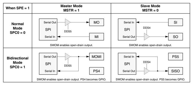
Figure 14-14. Normal Mode and Bidirectional Mode
