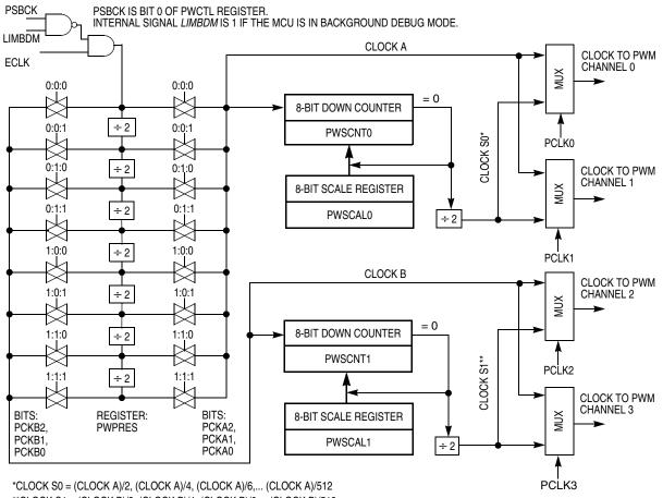
\*\*CLOCK S1 = (CLOCK B)/2, (CLOCK B)/4, (CLOCK B)/6,... (CLOCK B)/512
