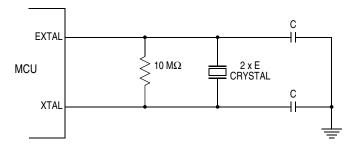
Figure 1-5. Common Crystal Connections
