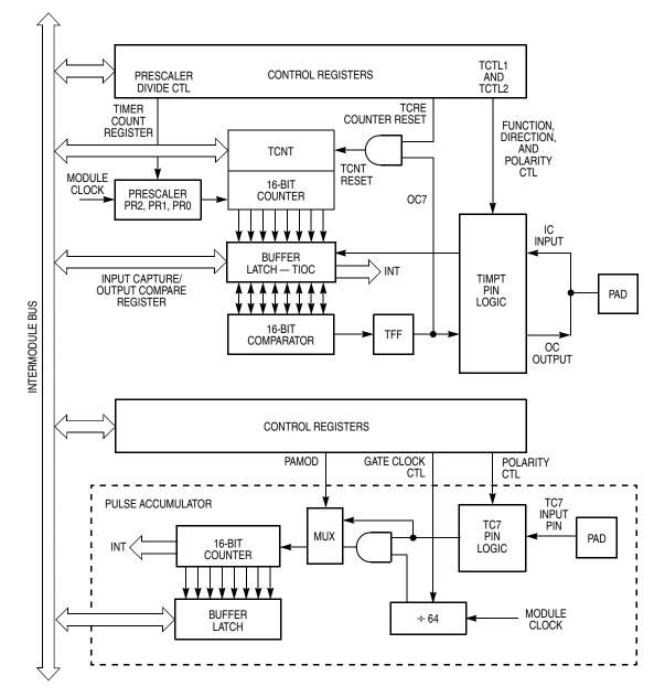
Figure 12-2. Timer Block Diagram
