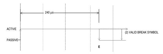
Figure 15-9. J1850 VPW Received BREAK Symbol Times
