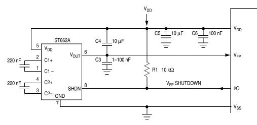
Figure 19-2. V<sub>FP</sub> Supply Circuit
