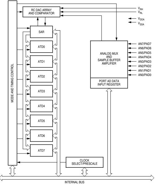
Figure 17-1. ATD Block Diagram
