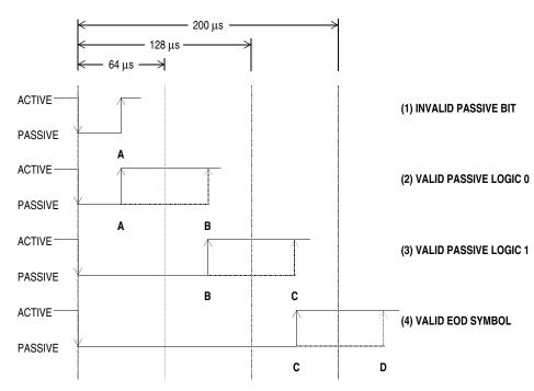
Figure 15-6. J1850 VPW Received Passive Symbol Times
