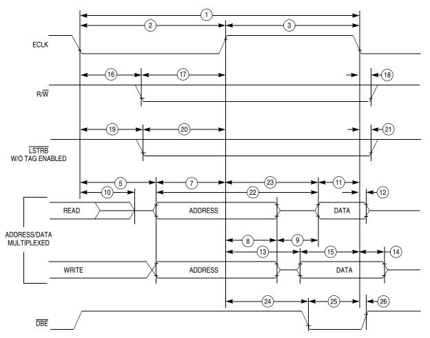
Note: Measurement points shown are 20% and 70% of  $V_{\text{DD}}$ .
