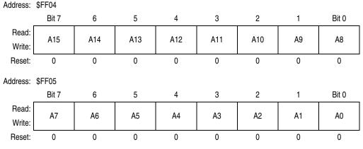
Figure 18-8. BDM Address Register (ADDRESS)
