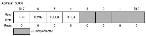
Figure 13-11. Timer System Control Register (TSCR)
