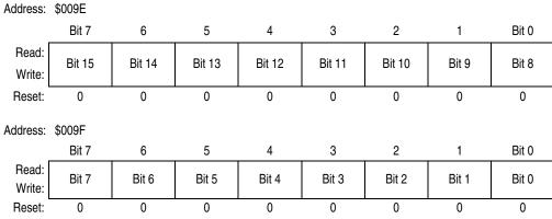
Figure 12-23. Timer Input Capture/Output Compare Register 7 (TC7)
