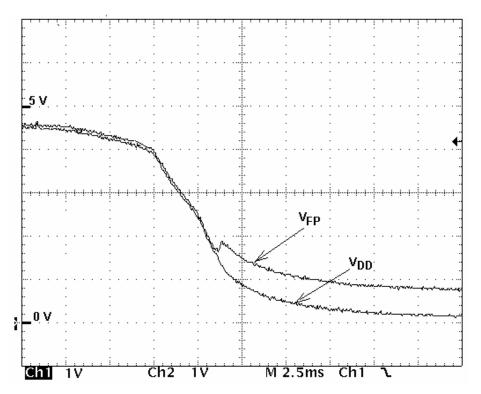
Figure 19-3. V<sub>FP</sub> Exceeding  $V_{DD}$  during Power-Down
