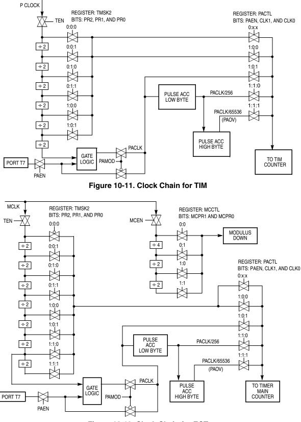
Figure 10-12. Clock Chain for ECT
