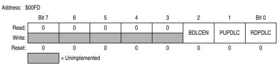
Figure 15-18. Port DLC Control Register (DLCSCR)
