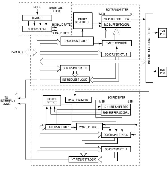
Figure 14-2. Serial Communications Interface Block Diagram
