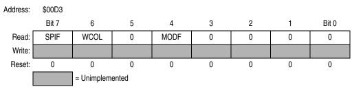
Figure 14-18. SPI Status Register (SP0SR)
