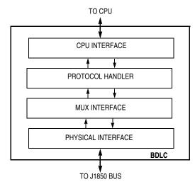
Figure 15-1. BDLC Block Diagram
