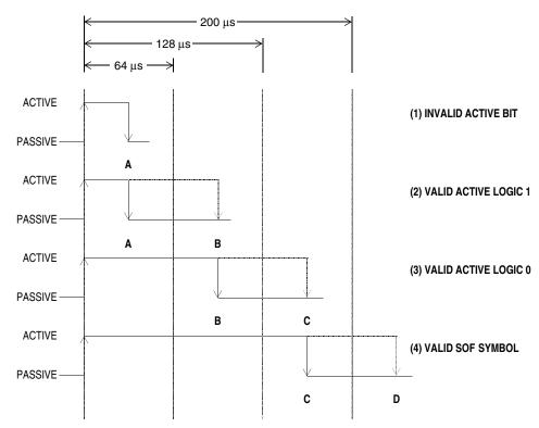
Figure 15-8. J1850 VPW Received Active Symbol Times
