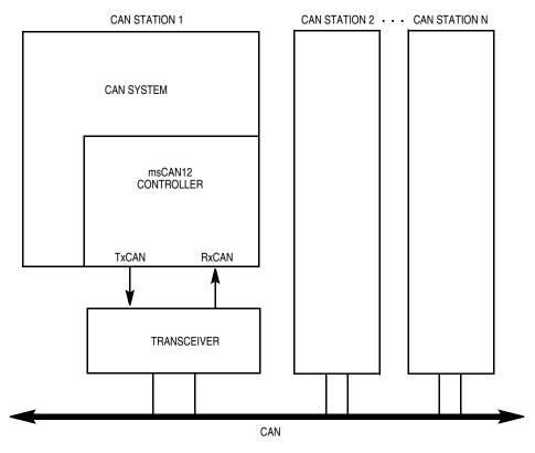
Figure 16-1. Typical CAN System with msCAN12
