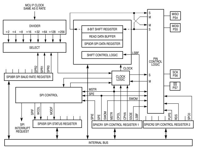
Figure 14-11. Serial Peripheral Interface Block Diagram
