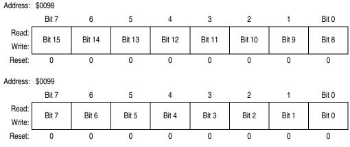
Figure 12-20. Timer Input Capture/Output Compare Register 4 (TC4)
