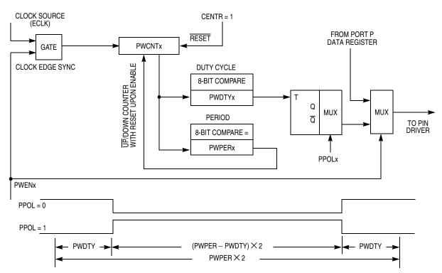
Figure 11-2. Block Diagram of PWM Center-Aligned Output Channel
