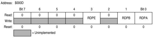
Figure 6-9. Reduced Drive of I/O Lines (RDRIV)
