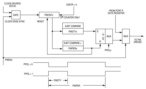
Figure 11-1. Block Diagram of PWM Left-Aligned Output Channel
