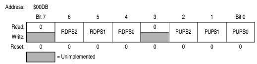
Figure 14-22. Pullup and Reduced Drive Register for Port S (PURDS)
