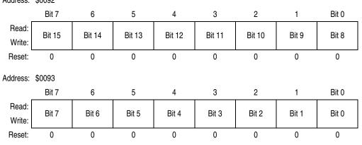
Figure 12-17. Timer Input Capture/Output Compare Register 1 (TC1)
