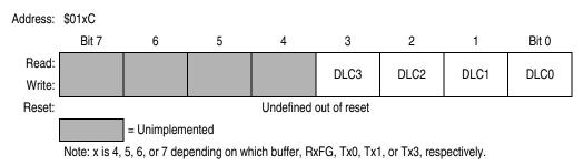
Figure 16-13. Data Length Register (DLR)
