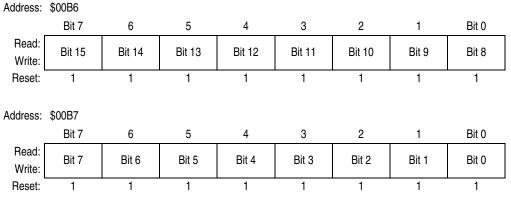
Figure 13-50. Modulus Down-Counter Count Registers (MCCNT)
