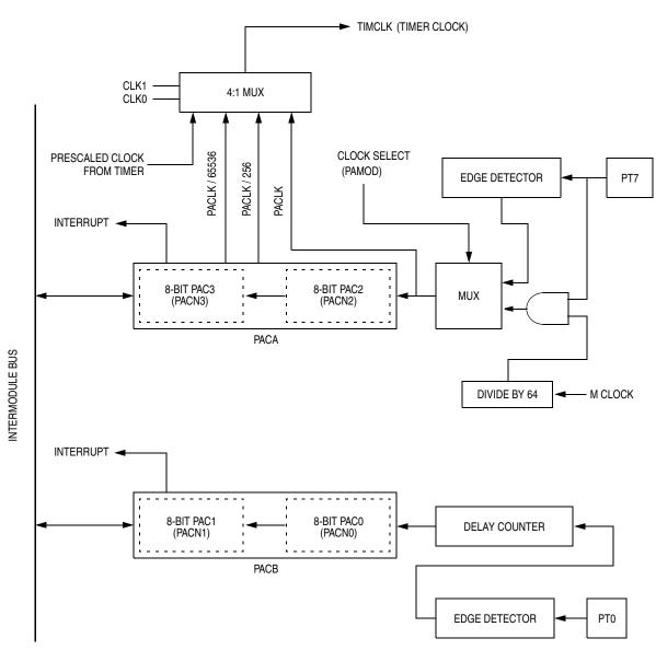
Figure 13-4. 16-Bit Pulse Accumulators Block Diagram
