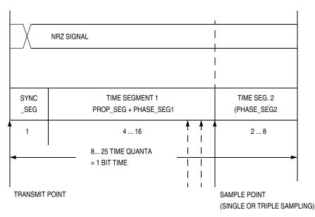
Figure 16-8. Segments within the Bit Time
