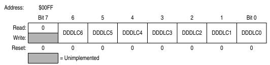
Figure 15-20. Port DLC Data Direction Register (DDRDLC)
