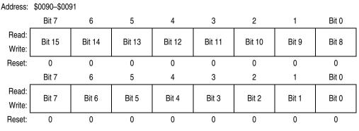
Figure 13-21. Timer Input Capture/Output Compare Register 0 (TC0)
