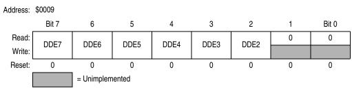
Figure 6-6. Port E Data Direction Register (DDRE)
