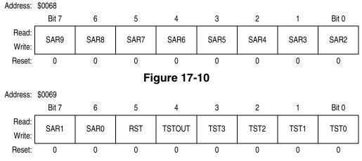
Figure 17-11. ATD Test Register (ATDSTAT)
