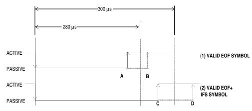
Figure 15-7. VPW Received Passive EOF and IFS Symbol Times
