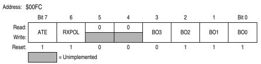
Figure 15-17. BDLC Analog Roundtrip Delay Register (BARD)
