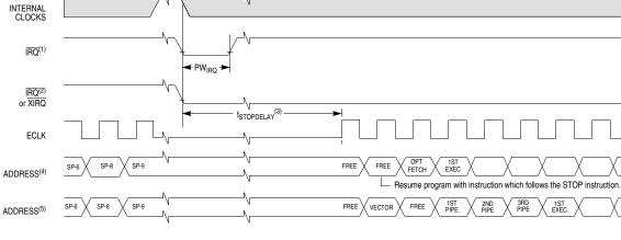
Notes: 1. Edge-sensitive  $\overline{IRQ}$  pin (IRQE bit = 1) 2. Level-sensitive  $\overline{IRQ}$  pin (IRQE bit = 0) 3.  $t_{\underline{STOPDELAY}} = 4098 t_{cyc}$  if DLY bit = 1 or 2  $t_{cyc}$  if DLY = 0. 4. XIRQ with X bit in CCR = 1. 5. IRQ or (XIRQ with X bit in CCR = 0)
