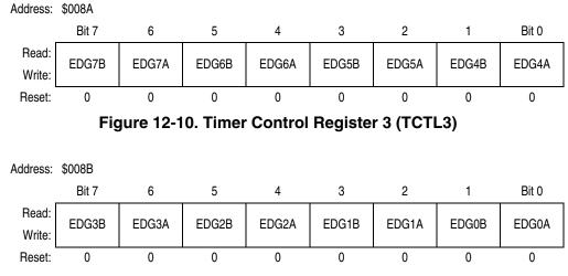
Figure 12-11. Timer Control Register 4 (TCTL4)
