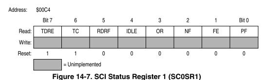
Read: Anytime; used in auto clearing mechanism
