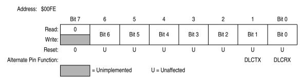
Figure 15-19. Port DLC Data Register (PORTDLC)
