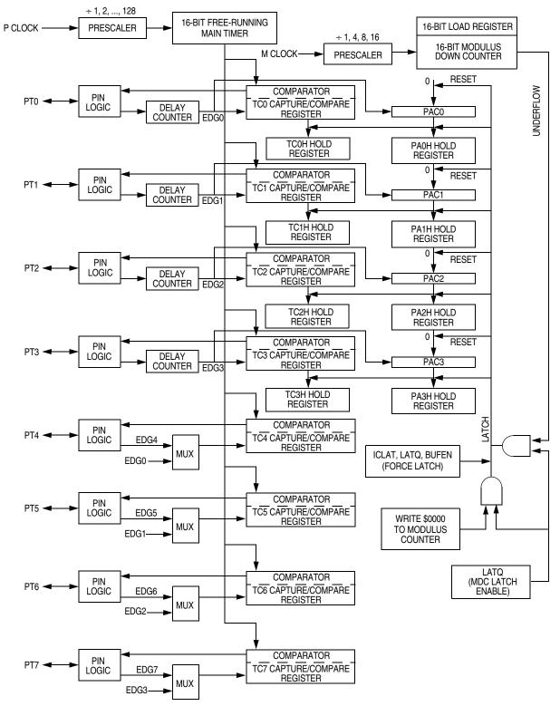
Figure 13-1. Timer Block Diagram in Latch Mode
