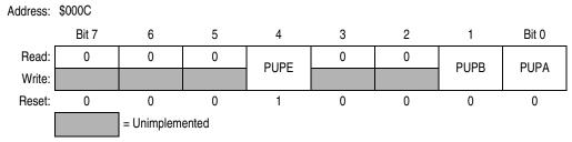
Figure 6-8. Pullup Control Register (PUCR)
