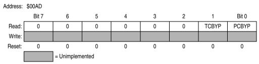
Figure 12-27. Timer Test Register (TIMTST)
