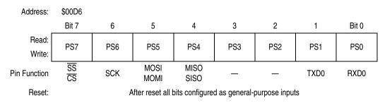
Figure 14-20. Port S Data Register (PORTS)
