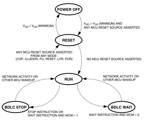
Figure 15-2. BDLC Operating Modes State Diagram
