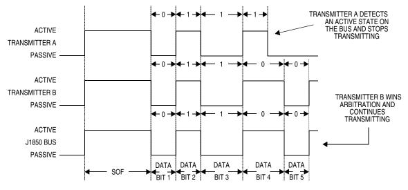
Figure 15-10. J1850 VPW Bitwise Arbitrations
