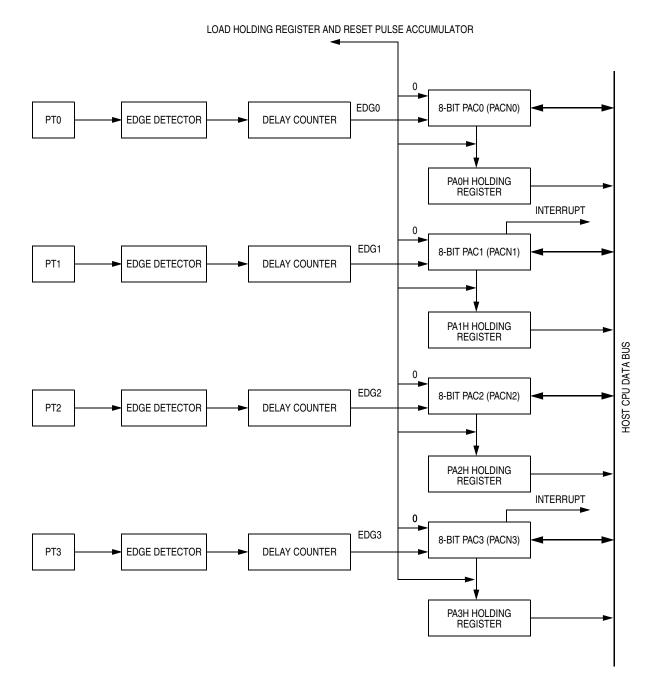
Figure 13-3. 8-Bit Pulse Accumulators Block Diagram
