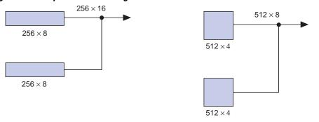
If necessary, all EABs in a device can be cascaded to form a single RAM block. EABs can be cascaded to form RAM blocks of up to 2,048 words without impacting timing. Altera's software automatically combines EABs to meet a designer's RAM specifications.
