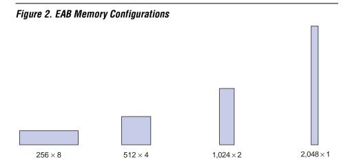
Larger blocks of RAM are created by combining multiple EABs. For example, two  $256 \times 8$  RAM blocks can be combined to form a  $256 \times 16$  RAM block; two  $512 \times 4$  blocks of RAM can be combined to form a  $512 \times 8$  RAM block. See Figure 3.
