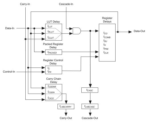
Figure 26. FLEX 10K Device IOE Timing Model
