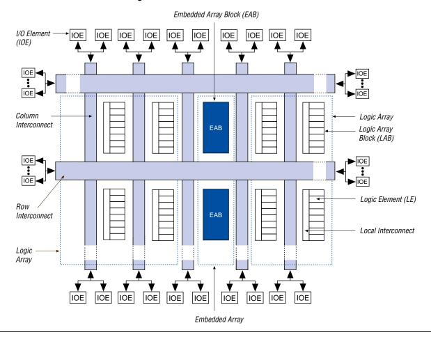
Figure 1. FLEX 10K Device Block Diagram
