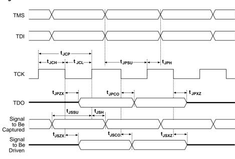
Table 16 shows the timing parameters and values for FLEX 10K devices.
