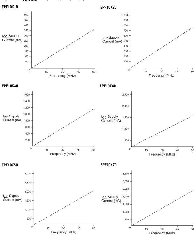
Figure 32. I<sub>CCACTIVE</sub> vs. Operating Frequency (Part 2 of 3)
