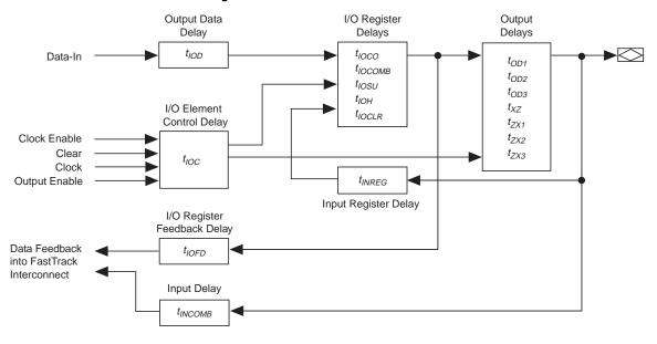
Figure 27. FLEX 10K Device EAB Timing Model
