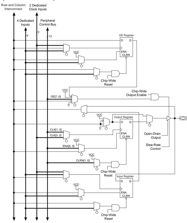
Each IOE selects the clock, clear, clock enable, and output enable controls from a network of I/O control signals called the peripheral control bus. The peripheral control bus uses high-speed drivers to minimize signal skew across devices; it provides up to 12 peripheral control signals that can be allocated as follows:
