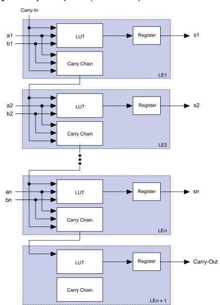
Figure 7. Carry Chain Operation (n-bit Full Adder)
