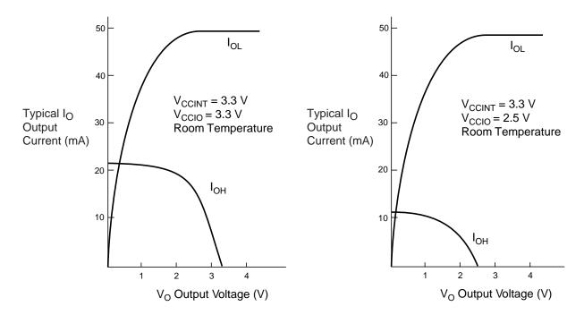
Figure 23. Output Drive Characteristics for EPF10K250A Device
