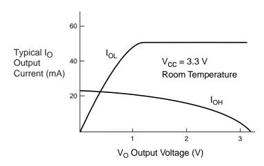
Figure 21. Output Drive Characteristics of EPF10K50V & EPF10K130V Devices
