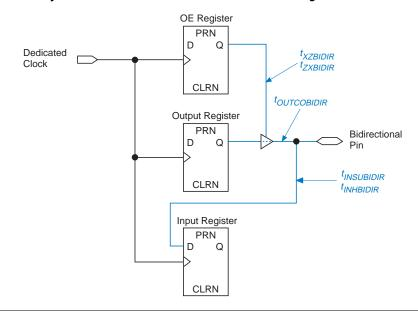
Figure 28. Synchronous Bidirectional Pin External Timing Model
