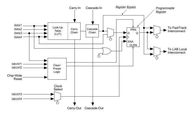
The programmable flipflop in the LE can be configured for D, T, JK, or SR operation. The clock, clear, and preset control signals on the flipflop can be driven by global signals, general-purpose I/O pins, or any internal logic. For combinatorial functions, the flipflop is bypassed and the output of the LUT drives the output of the LE.
