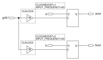
Figure 17. Enabling ClockLock & ClockBoost in the Same Design
