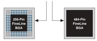
256-Pin FineLine BGA Package (Reduced I/O Count or Logic Requirements) 484-Pin FineLine BGA Package (Increased I/O Count or Logic Requirements)
