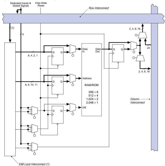
Figure 4. FLEX 10K Embedded Array Block
