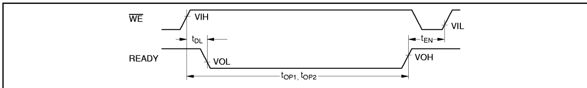
Figure 29 READY Timing (When the READY Output Is Always Available)
