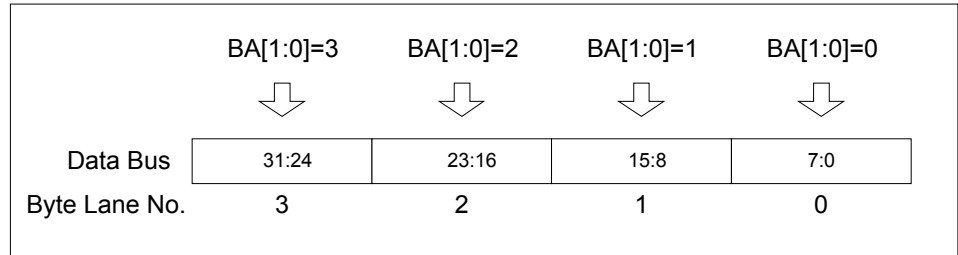
Figure 3-2. Little-Endian Mode Addressing
