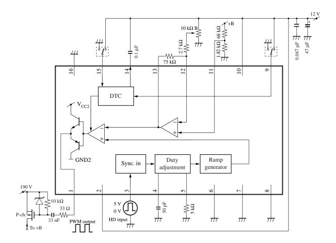
Note) When both of the pin 4 and the pin 5 are open, minimum pulse width of PWM output is  $2.0 \ \mu s$ .
