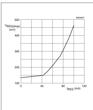
Fig.16 Dropout voltage as a function of the output current.
