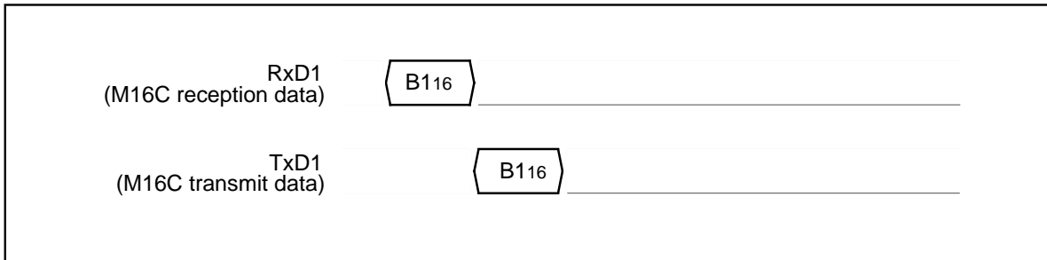
Figure 1.29.40. Timing of baud rate 19200
