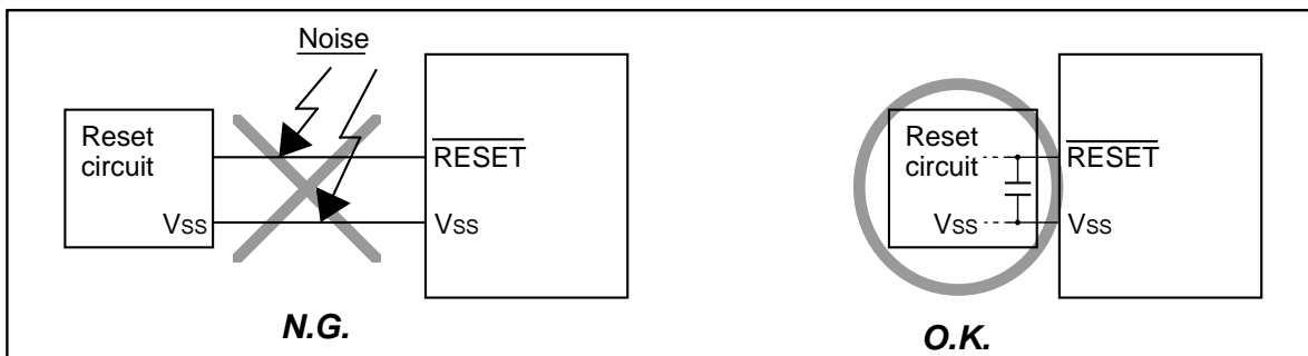
Figure 1.1.2. Wiring for RESET pin
