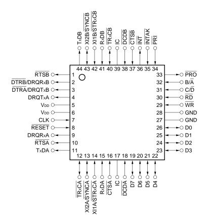
IC: Internally Connected (Leave this pin unconnected)
