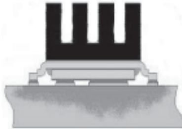
⑨ Mounted on minimum footprint full size board with metalized back and with small clip heatsink. (still air)
