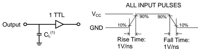
1. Including jig and scope capacitance.
