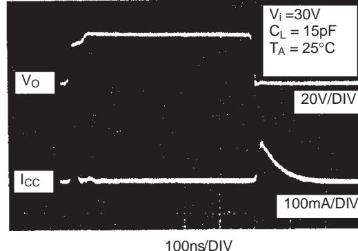
**Figure 14:** Oscillator and Output Waveforms.
