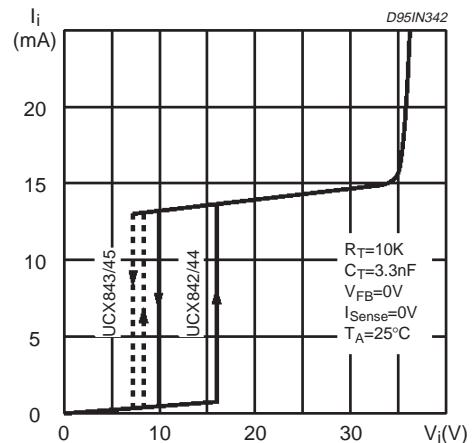
**Figure 13:** Output Cross Conduction
