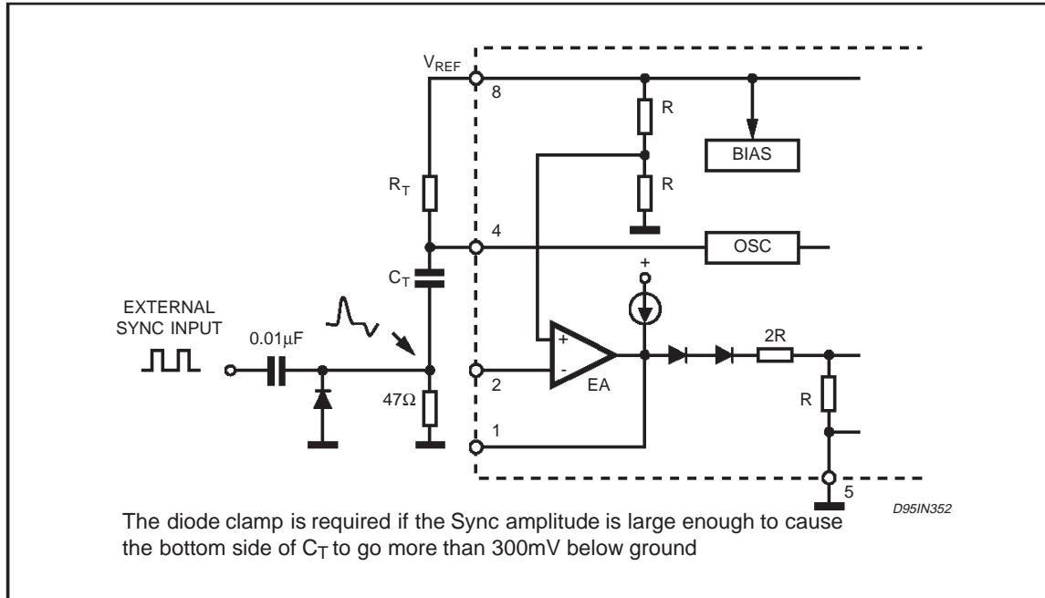
**Figure 23:** External Duty Cycle Clamp and Multi Unit Synchronization.
