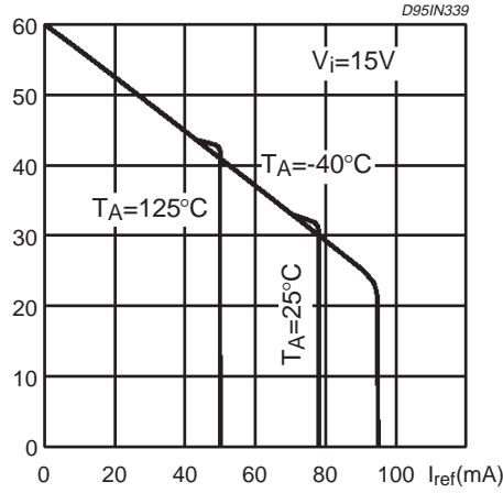
**Figure 5:** Maximum Output Duty Cycle vs. Timing Resistor.
