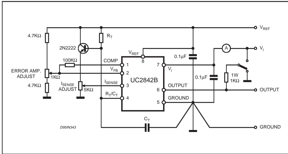
High peak currents associated with capacitive loads necessitate careful grounding techniques. Timing and bypass capacitors should be connected close
