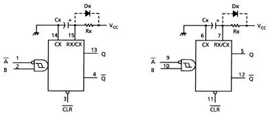
Note 1: Cx, Rx, Dx are external capacitor, resistor, and diode, respectively.
