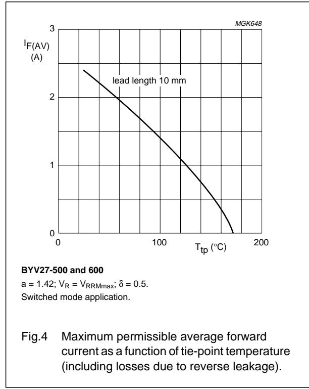
Fig.4 Maximum permissible average forward current as a function of tie-point temperature (including losses due to reverse leakage).
