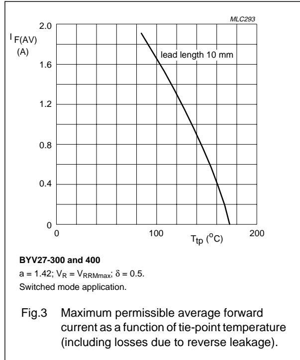
Fig.3 Maximum permissible average forward current as a function of tie-point temperature (including losses due to reverse leakage).
