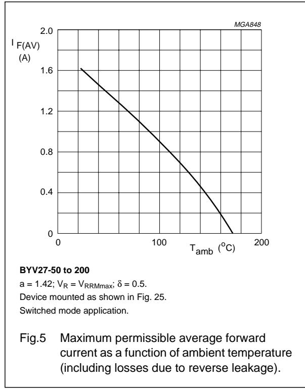
Fig.5 Maximum permissible average forward current as a function of ambient temperature (including losses due to reverse leakage).
