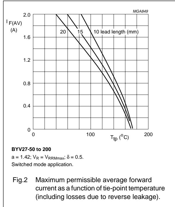
Fig.2 Maximum permissible average forward current as a function of tie-point temperature (including losses due to reverse leakage).
