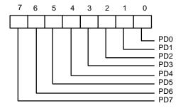
When accesses are made to any EPP data port, the contents of DB0-DB7 are buffered (non-inverting) and output to the ports PD0-PD7 during a write operation. The leading edge of  $\overline{\text{IOW}}$  causes
