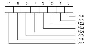
The contents of DB0-DB7 are buffered (non-inverting) and output to ports PD0-PD7 during a write operation. The leading edge of IOW causes an EPP address write cycle to be performed, and the trailing edge of IOW latches the data for the duration of the EPP write cycle.
