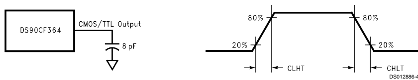
FIGURE 4. DS90CF364 (Receiver) CMOS/TTL Output Load and Transition Times
