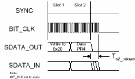
AC-Link low power mode timing diagram
