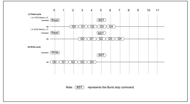
Timing Chart of Burst Stop Cycle (Precharge Command)
