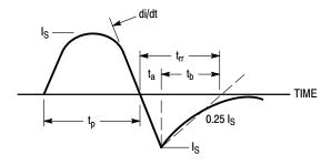
Figure 15. Diode Reverse Recovery Waveform
