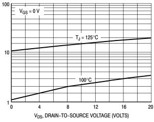
Figure 6. Drain-to-Source Leakage Current versus Voltage
