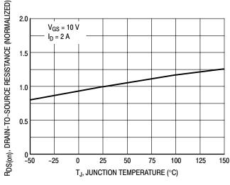
Figure 5. On–Resistance Variation with Temperature
