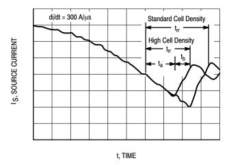
Figure 11. Reverse Recovery Time (t<sub>rr</sub>)
