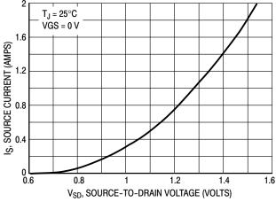
Figure 10. Diode Forward Voltage versus Current
