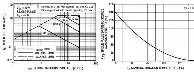
Figure 12. Maximum Rated Forward Biased Safe Operating Area
