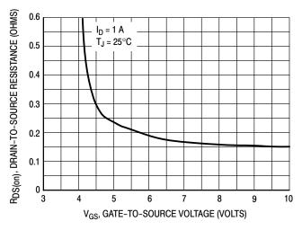
Figure 3. On–Resistance versus Gate–to–Source Voltage
