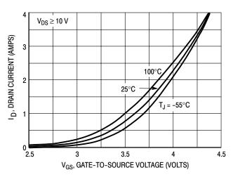
Figure 2. Transfer Characteristics
