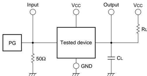
(1) Characteristics of pulse generator (PG) (10% to 90%)
