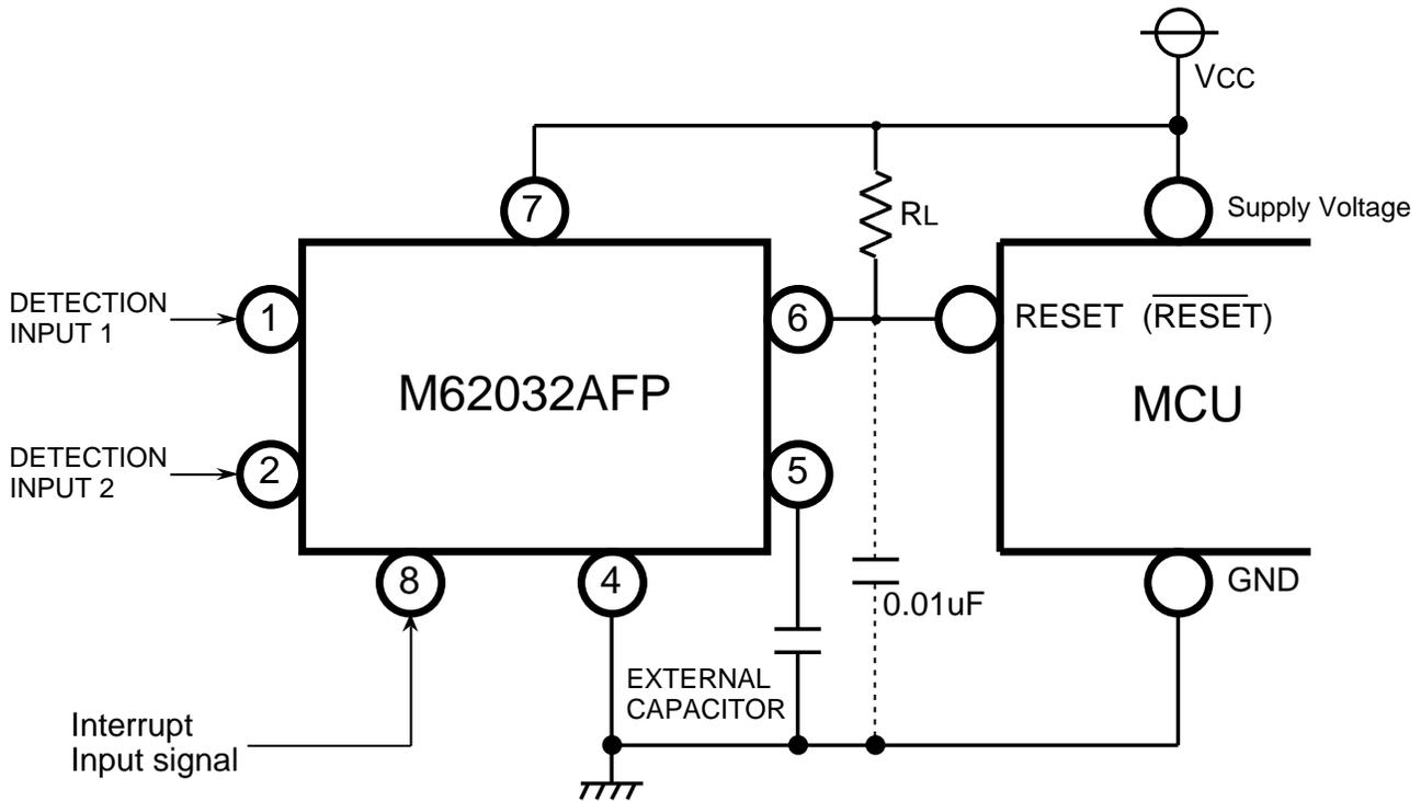
\* A forced reset signal (high) into pin 8 from outside can reset this IC (low output) regardless of input signals to pins 1 and 2.
