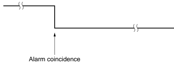
Fig. 2 “H” → “L” Output Waveform
