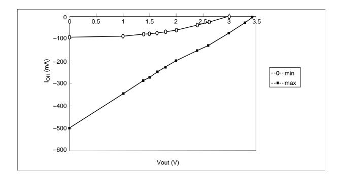
**DC Characteristics** (Ta = 0 to +70°C,  $V_{CC}$ ,  $V_{CC}Q = 3.3 \text{ V} \pm 0.3 \text{ V}$ ,  $V_{SS}$ ,  $V_{SS}Q = 0 \text{ V}$ ) (HM5264165F)
