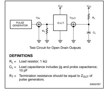
Figure 21. Test circuit
