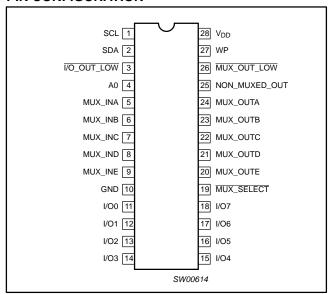
Figure 1. Pin configuration
