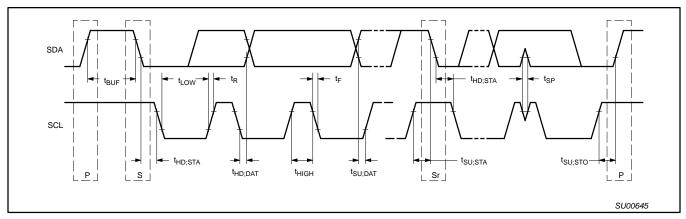
Figure 19. Definition of timing
