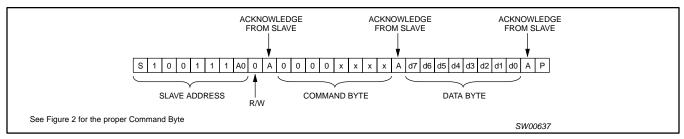
Figure 9. I<sup>2</sup>C write for GPIO registers
