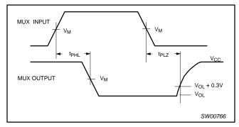
Figure 20. Open drain output enable and disable times
