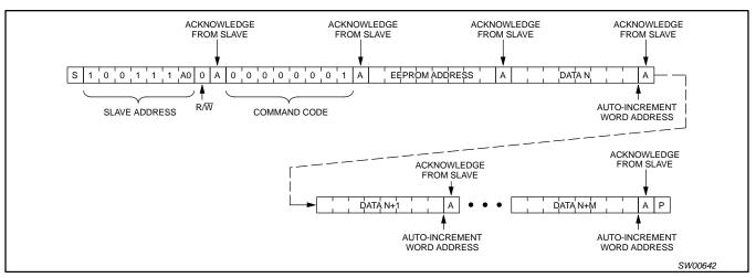
Figure 14. I<sup>2</sup>C page write operation to 256 byte EEPROM; M bytes where M ≤ 15
