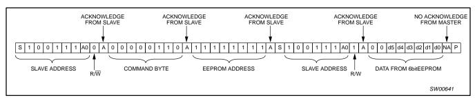
Figure 13. I<sup>2</sup>C read of 6-bit EEPROM
