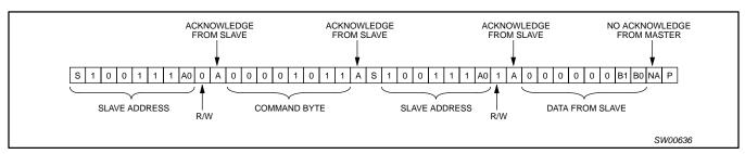
Figure 8. I<sup>2</sup>C read for MUXCNTRL register
