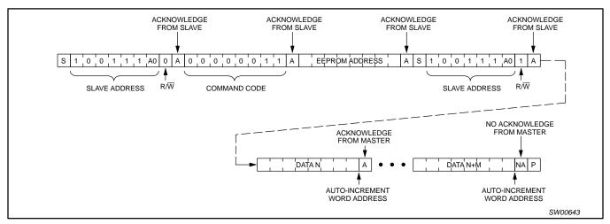
Figure 15. I<sup>2</sup>C read operation from 256 byte EEPROM; M bytes where M ≥ 1
