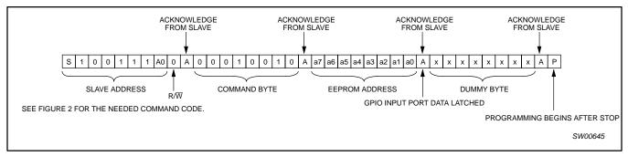
Figure 17. Read from GPIO Input Port Register and write to 256 byte EEPROM
