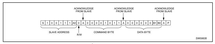
Figure 7. I<sup>2</sup>C write for MUXCNTRL register
