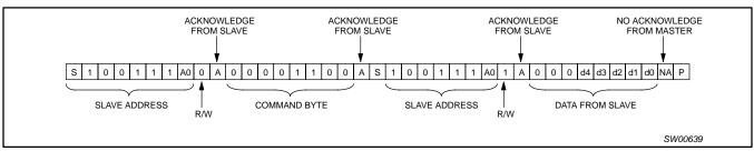
Figure 11. I<sup>2</sup>C read of MUX\_INx inputs
