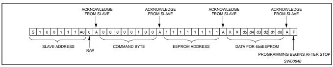
Figure 12. I<sup>2</sup>C write of 6-bit EEPROM
