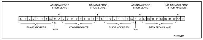
Figure 10. I<sup>2</sup>C read for GPIO registers
