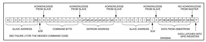
Figure 16. Read from 256 byte EEPROM and write to GPIO registers
