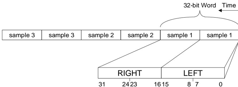
**Figure 16. 16-bit Stereo, Signed Little Endian Audio Data**
