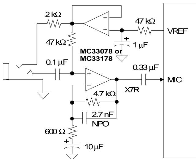
**Figure 21. Microphone Input**
