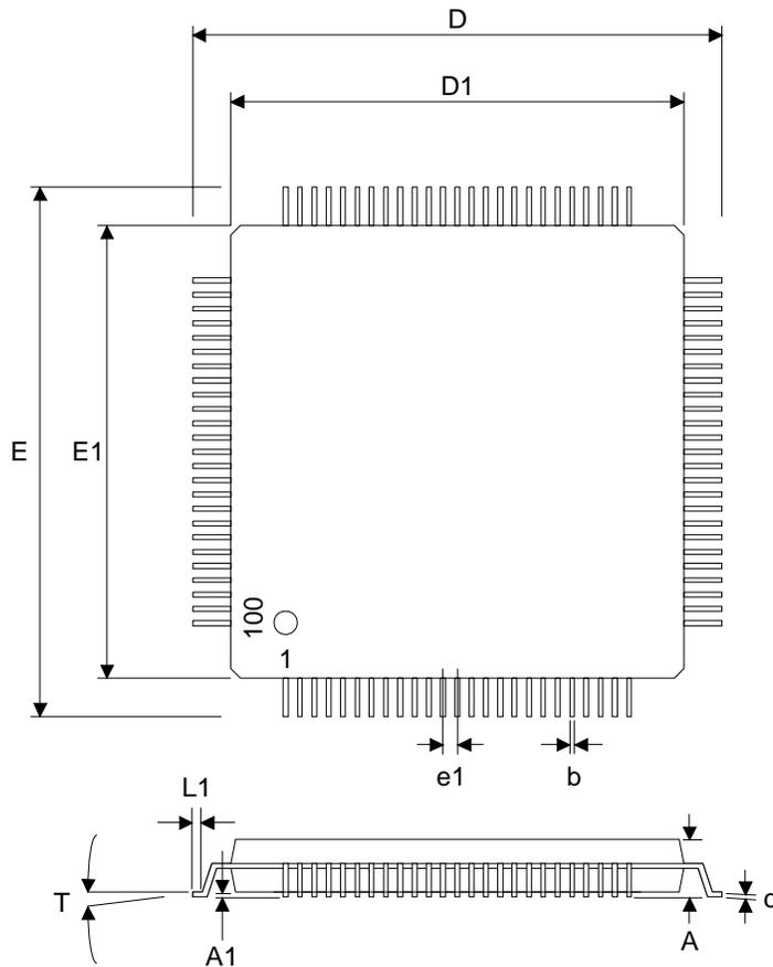
**100-pin TQFP - Package Code 'Q'**
