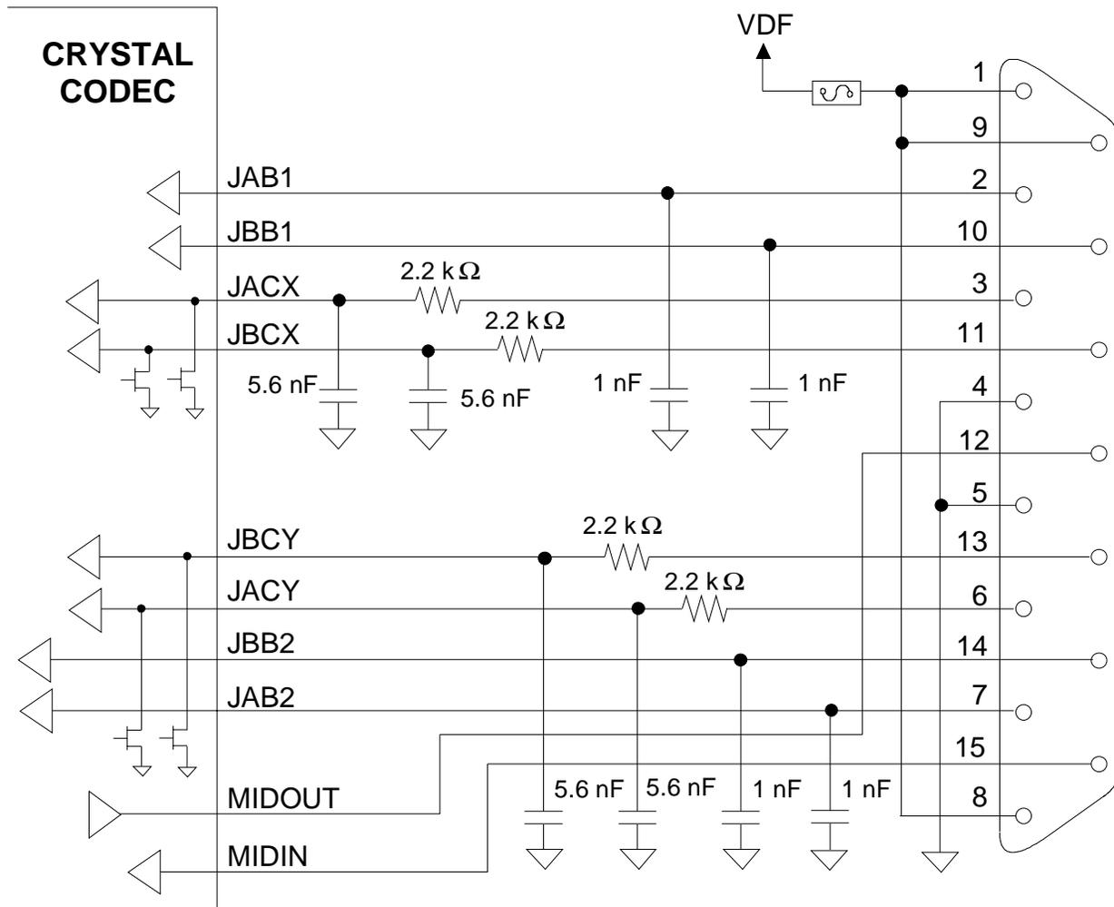
Figure 5. Joystick Logic
