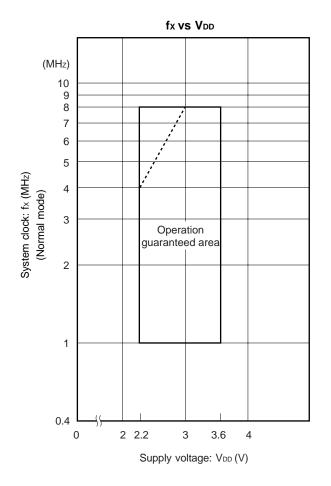
**Remark** The region indicated by the broken line in the above figure is the guaranteed operating range in the high-speed mode.
