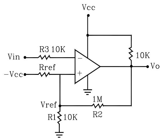
**FIGURE 3 - NON-INVERTING COMPARATOR WITH HYSTERESIS**
