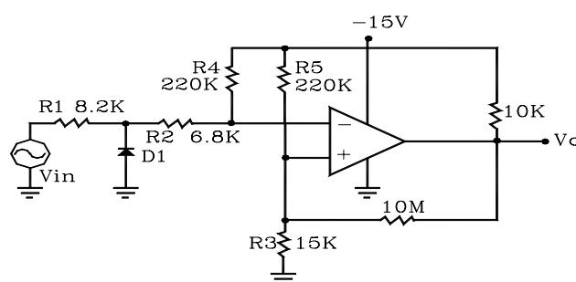
**FIGURE 10 - ZERO CROSSING DETECTOR
