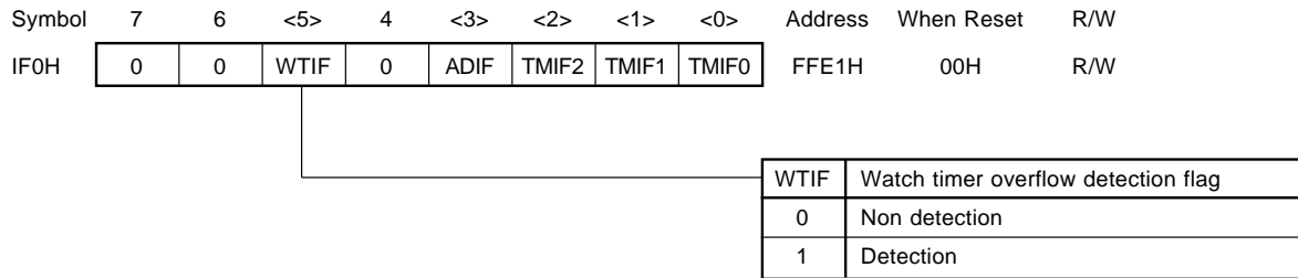
Figure 18-18. Interrupt Request Flag Register 0H Format
