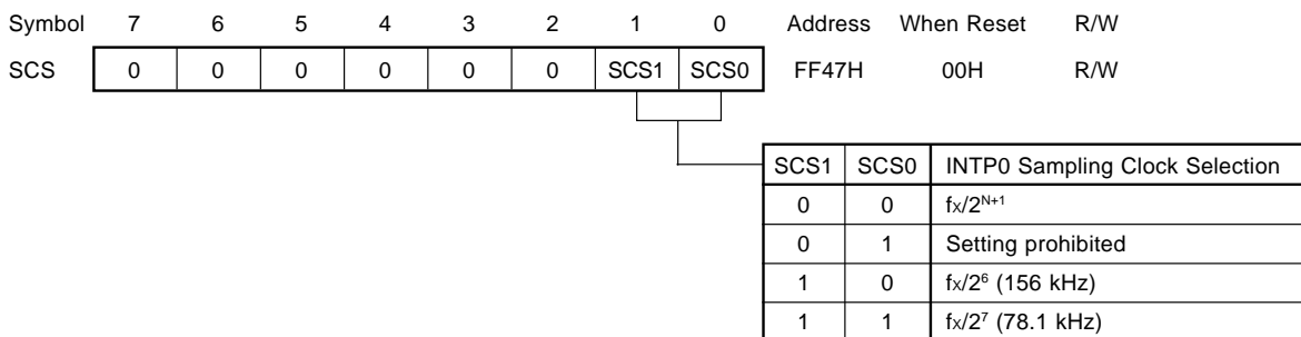
Figure 8-9. Sampling Clock Select Register Format
