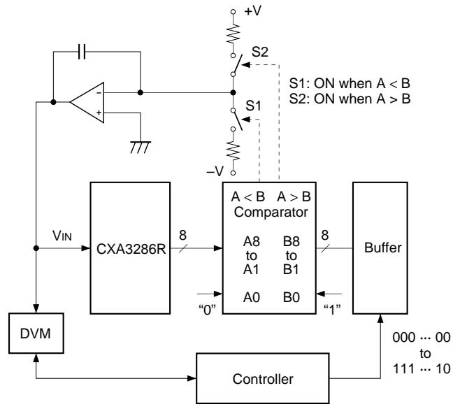
**Aperture Jitter Measurement Method**
