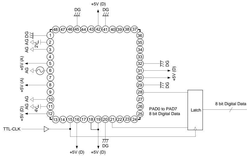
**Application Circuit 2      DMUX Mode TTL I/O (When a single power supply is used)**
