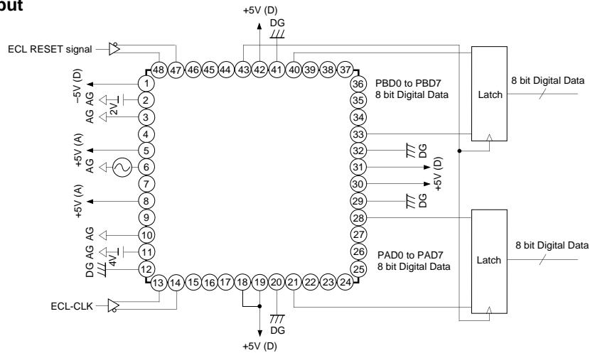
**(2) DMUX PECL input**
