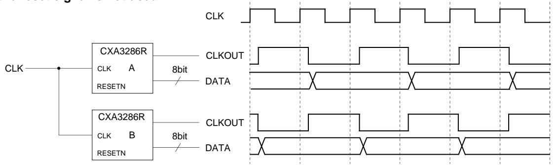
**When the reset signal is used**
