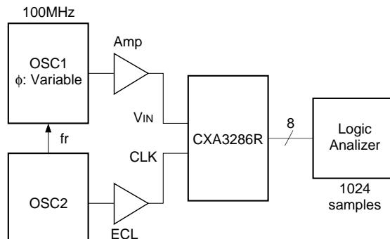
**Integral Linearity Error Measurement Circuit****Differential Linearity Error Measurement Circuit**
