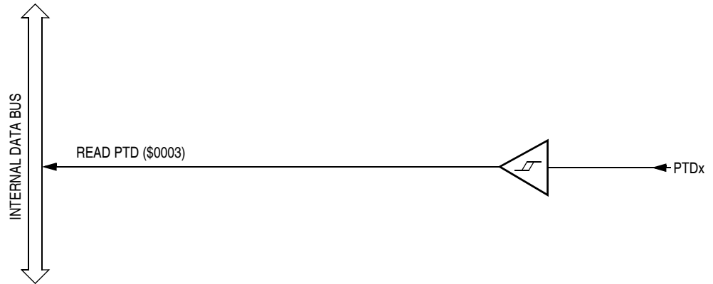
Figure 15-12. Port D Input Circuit
