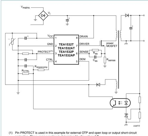
protection. Slope compensation is determined by the value of  $R_{\text{slopecomp}}$ .
