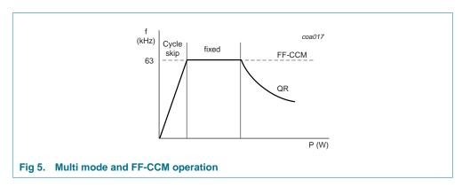
In QR mode, the next converter stroke is started only after demagnetization of the transformer current (zero current switching), while the drain voltage has reached the lowest voltage to minimize switching losses (green function). The primary resonant circuit of primary inductance and drain capacitor ensures this quasi-resonant operation. The design can be optimized in such a way that zero voltage switching can extend over most of the universal mains range.
