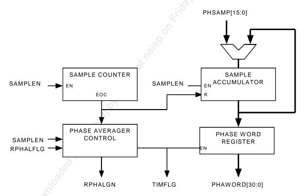
Although referred to as an averaging process, it is truly an accumulation process. It retains full resolution, i.e. no division is performed on the accumulated value. The Phase Word includes an integer and a fractional part. The number of averaging samples sets the size of the fractional part.
