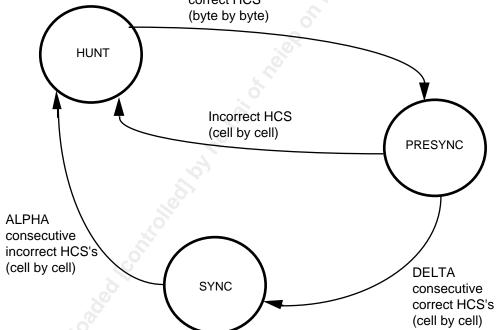
The values of ALPHA and DELTA determine the robustness of the delineation process. ALPHA determines the robustness against false misalignments due to bit errors. DELTA determines the robustness against false delineation in the synchronization process. ALPHA is chosen to be 7 and DELTA is chosen to be 6. These values result in an average time to delineation of 33.66 µs for the STS-3c (STM-1) rate.
