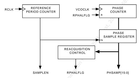
Successive reading of the value obtained, referred to as phase sample (PHSAMP), can be used to calculate the phase relation between both clocks. Both the Reference Counter and the Phase Counter are programmable counters and are set to have equal cycle period. Therefore, if VCOCLK is locked to RCLK, successive readings of the phase sample would be equal. The phase sample value would increase or decrease depending if VOCLK is faster or slower that RCLK.
