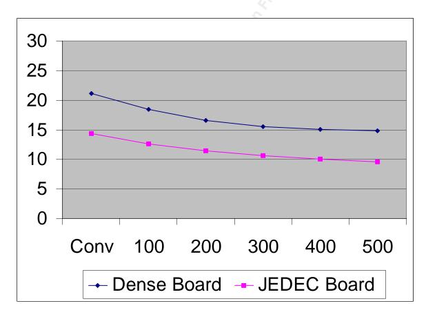
The junction temperature (Tj) is less than 105°C for a ambient temperature (Ta) of 60°C and a 300LFM of airflow. The device must operate at Ta=70°C with 100LFM and must not be damaged with Ta=70°C and no airflow. This assumes a dense board and a ThetaJA of 16.
