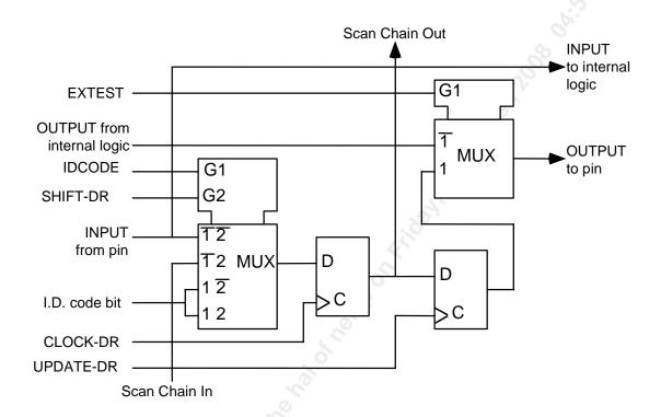
Figure 17: Layout of Output Enable and Bidirectional Cells
