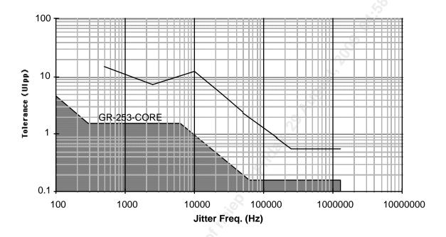
Note that for frequencies below 300 Hz, the jitter tolerance is greater than 15 Ulpp; 15 Ulpp is the maximum jitter tolerance of the test equipment. Also note that the dip in the tolerance curve between 300 Hz and 10 kHz is due to the S/UNI-TETRA's internal clock difference detector: if the recovered clock drifts beyond 488 ppm of the reference, the PLL locks to the reference clock.
