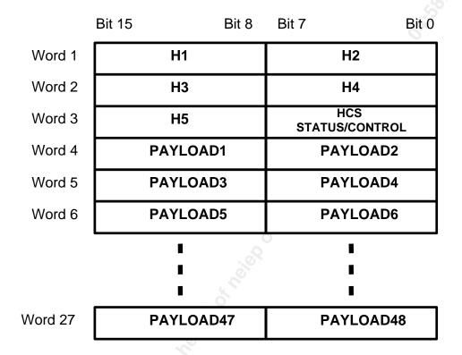
Bit 15 of each word is the most significant bit (which corresponds to the first bit transmitted or received). The header check sequence octet (HCS) is passed through this structure. The start of cell indication input and output (TSOC and RSOC) are coincident with Word 1 (containing the first two header octets). Word 3 of this structure contains the HCS octet in bits 15 to 8.
