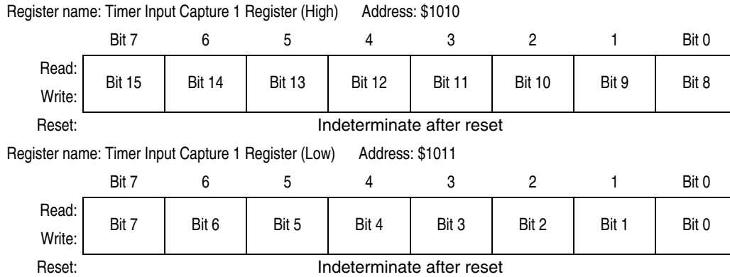
Figure 9-4. Timer Input Capture 1 Register Pair (TIC1)
