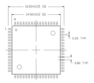
DIMENSIONS IN MILLIMETERS LEAD COPLANARITY 0.102 MAX.
