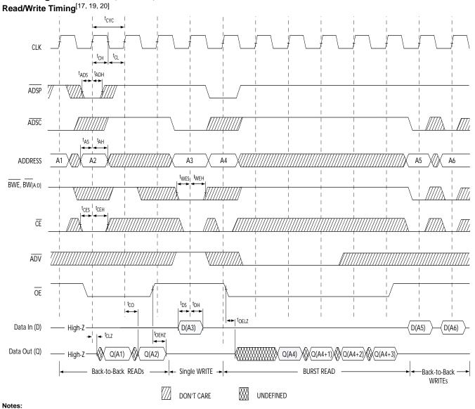
19. The data bus (Q) remains in Tri-State following a WRITE cycle unless a new read access is initiated by ADSP or ADSC-20. GW is HIGH-
