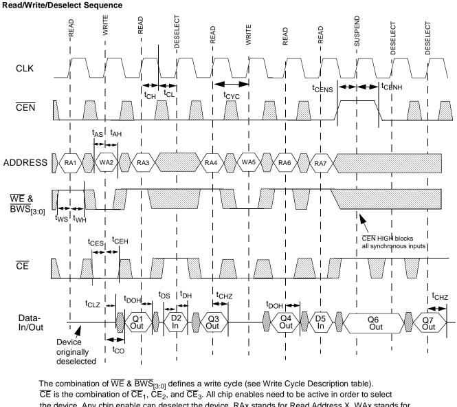
the device. Any chip enable can deselect the device. RAx stands for Read Address X, WAx stands for Write Address X, Dx stands for Data-in for location X, Qx stands for Data-out for location X. ADV/LD held LOW. OE held LOW.
