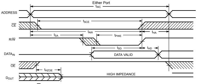
Write Cycle No. 2 (R/ $\overline{W}$  Three-States Data I/Os—Either Port)<sup>[16, 23]</sup>
