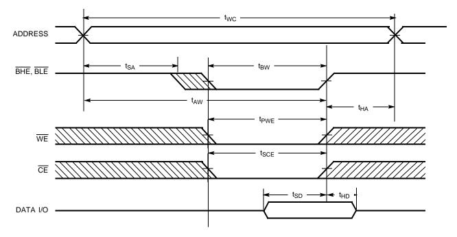
Notes: 12. Data I/O is high impedance if  $\overline{OE}$  or  $\overline{BHE}$  and/or  $\overline{BLE} = V_{IH}$ . 13. If  $\overline{CE}$  goes HIGH simultaneously with  $\overline{WE}$  going HIGH, the output remains in a high-impedance state.
