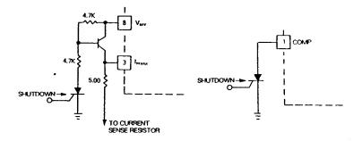
Shutdown of the DBL3842 can be accomplished by two methods; either raise pin3 above 1V or pull pin1 below a voltage two diodes drops above ground. Either method causes the output of the PWM comparator to be high (refer to
