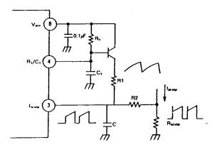
A fration of the oscillator ramp can be resistively summed with the current sense signal to provide slope compensation for coverters requiring duty cycle over 50%. Note that capacitor C, forms a filter with R2 to supress the leading edge switch spikes.
