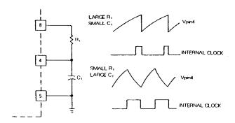
The oscillator frequency is programmed by the values selected for the timing components Rt and Ct. Ct is charged from 5V. Vref, through resistor Rt to approximately 2.8V and discharged to 1.2V by an internal current sink.
