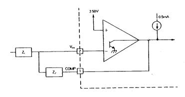
Error amp output(Pin1) is provided for external loop compensation and error amp can source or sink up to 0.5mA. The non—inverting input is internally biased at 2.5V and is not pinned out.
