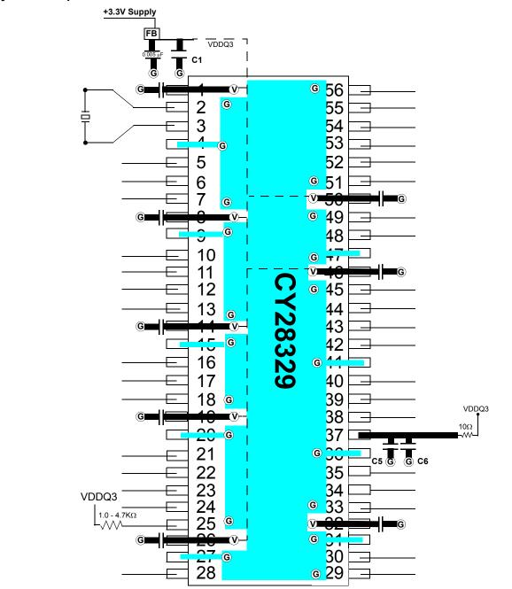
FB = Dale ILB1206 - 300 or 2TDKACB2012L-120 or 2 Murata BLM21B601S Ceramic Caps C1 = 10–22  $\mu$ F C2 = 0.005  $\mu$ F C5 = 0.1  $\mu$ F C6 = 10  $\mu$ F G = VIA to GND plane layer V =VIA to respective supply plane layer Note: Each supply plane or strip should have a ferrite bead and capacitors
