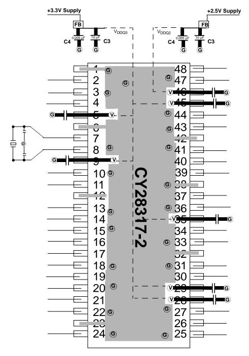
$\label{eq:FB} \begin{array}{l} \mbox{FB} = \mbox{Dale ILB1206} - 300 \; (300\Omega @ 100 \mbox{ MHz}) \; \mbox{or TDK ACB2012L-120} \\ \mbox{Ceramic Caps } C3 = 10{-}22 \; \mbox{$\mu$F$} & \mbox{C4} = 0.005 \; \mbox{$\mu$F$} \\ \mbox{C6} = 0.01 \; \mbox{$\mu$F$} \end{array}$
