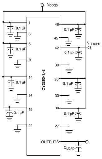
Note: All Capacitors must be placed as close to the pins as is possible
